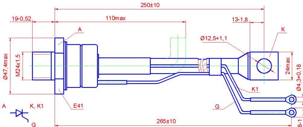
Tightening torque : 40 ÷ 60 Nm
